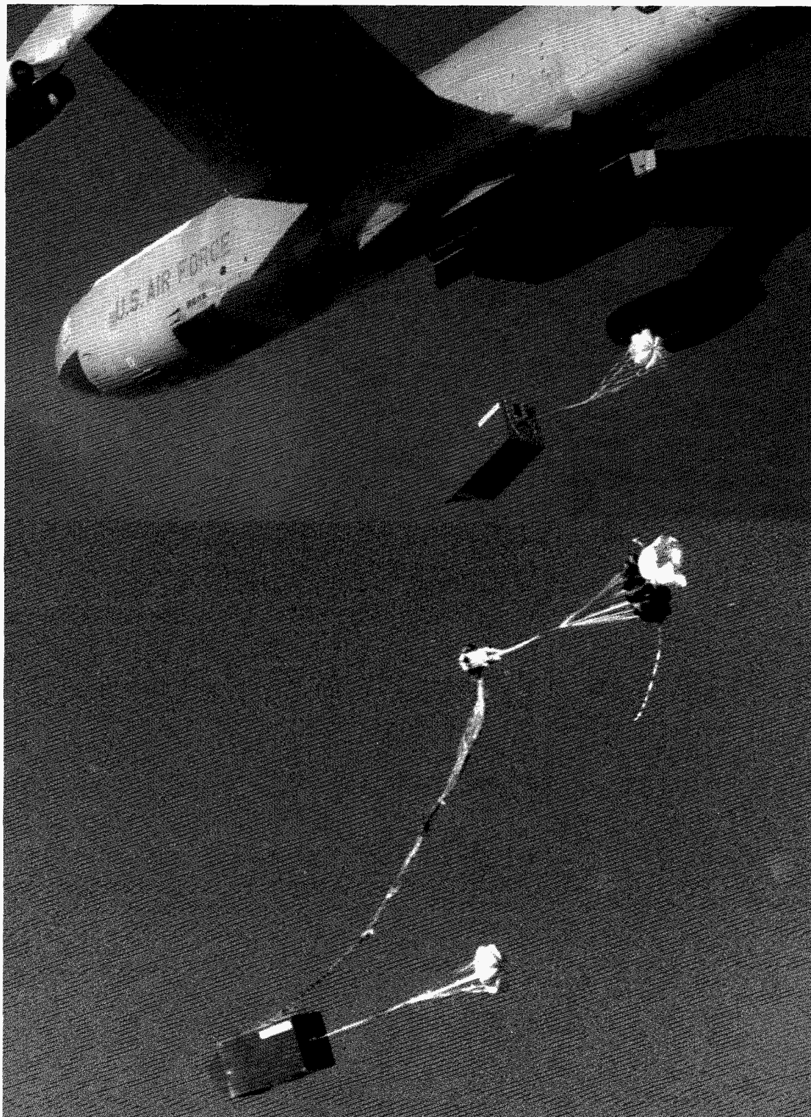
Parachute Development Testing. The F-111 PTV (Parachute Test Vehicle) testing parachutes for a crew escape capsule.
