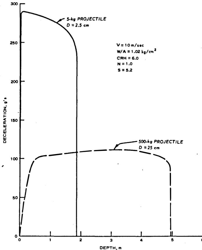
Figure 5. Comparison of calculated deceleration records in hypothetical soil target for impact velocity of 100 m/sec
