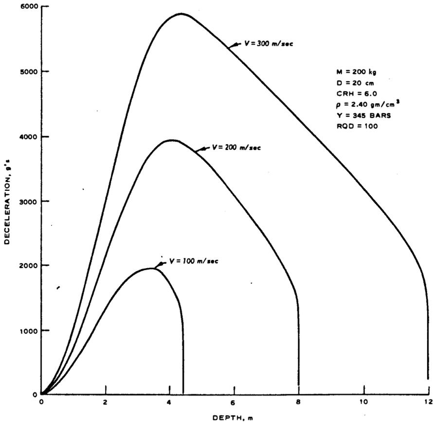
Figure 9. Calculated deceleration curves for 5000-psi concrete
