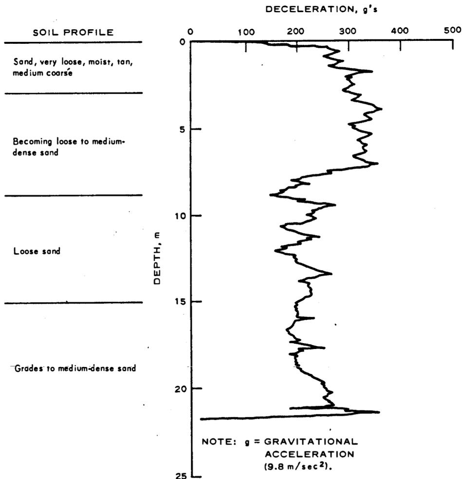
Figure 2. Measured deceleration record in moist sand
