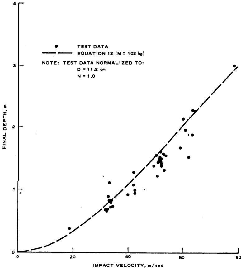
Figure 3. Correlation of TTR penetration data with Equation 12 for empirical determination of  $\alpha$  and  $\beta$
