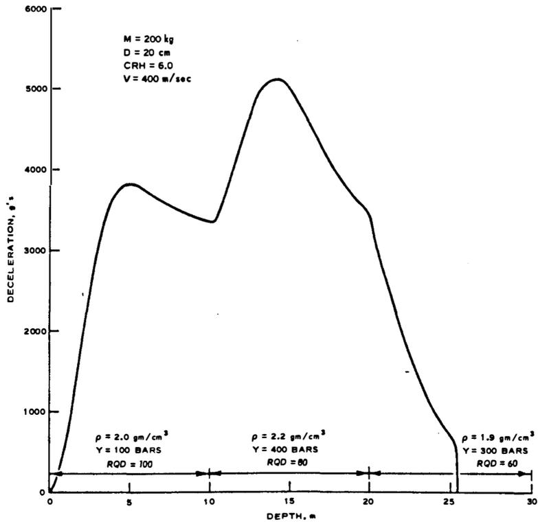
Figure 12. Calculated deceleration record for a hypothetical three-layer rock target
