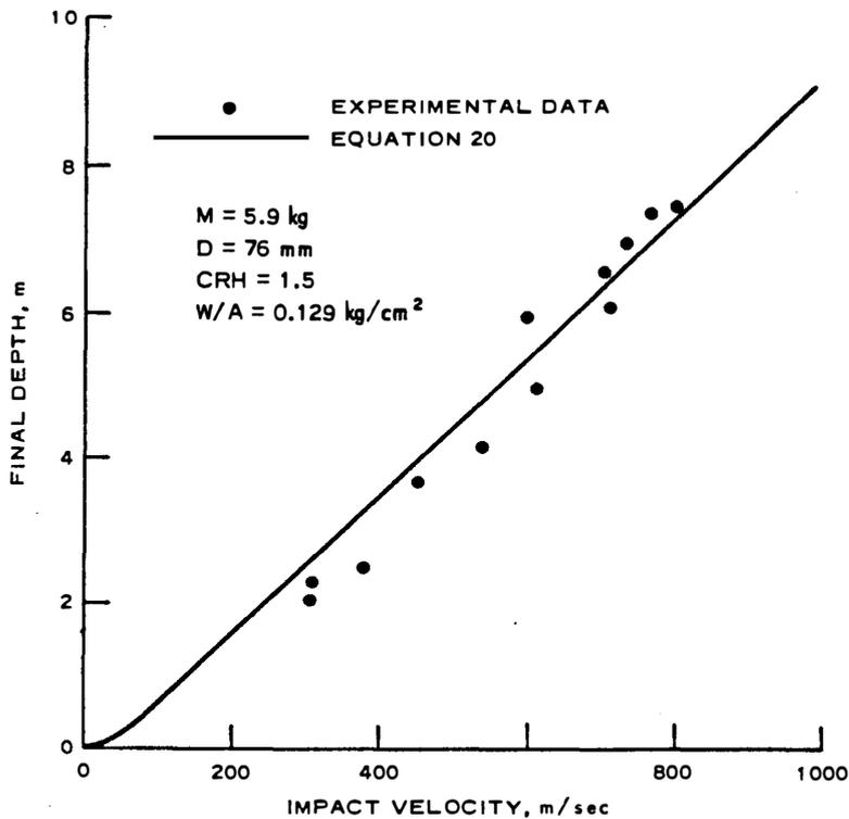
Figure 7. Correlation of penetration data for 5000-psi concrete with Equation 20 for empirical determination of  $a'$  and  $b'$
