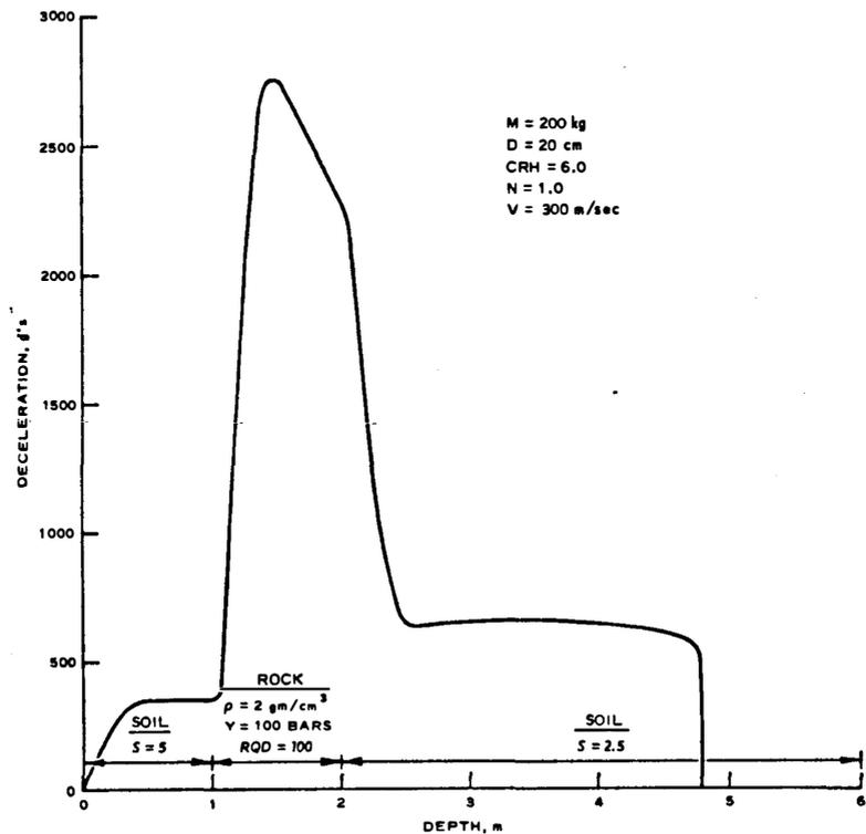
Figure 13. Calculated deceleration record for a hypothetical soil/rock/soil target
